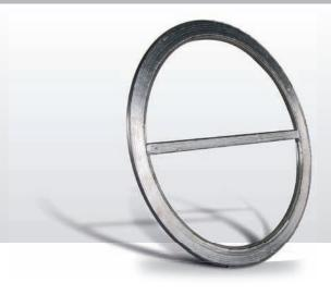
The Change gasket is manufactured with proprietary equipment, using a 5-times thicker metal spiral and a unique laser welding process that penetrates completely through the winding, so it requires no inner or outer ring and is easy to handle and install as a double-jacketed gasket. It's proven to perform without fail at least 60% longer than any other heat exchanger gasket – spiral wound, double jacketed, corrugated or kammprofile.
